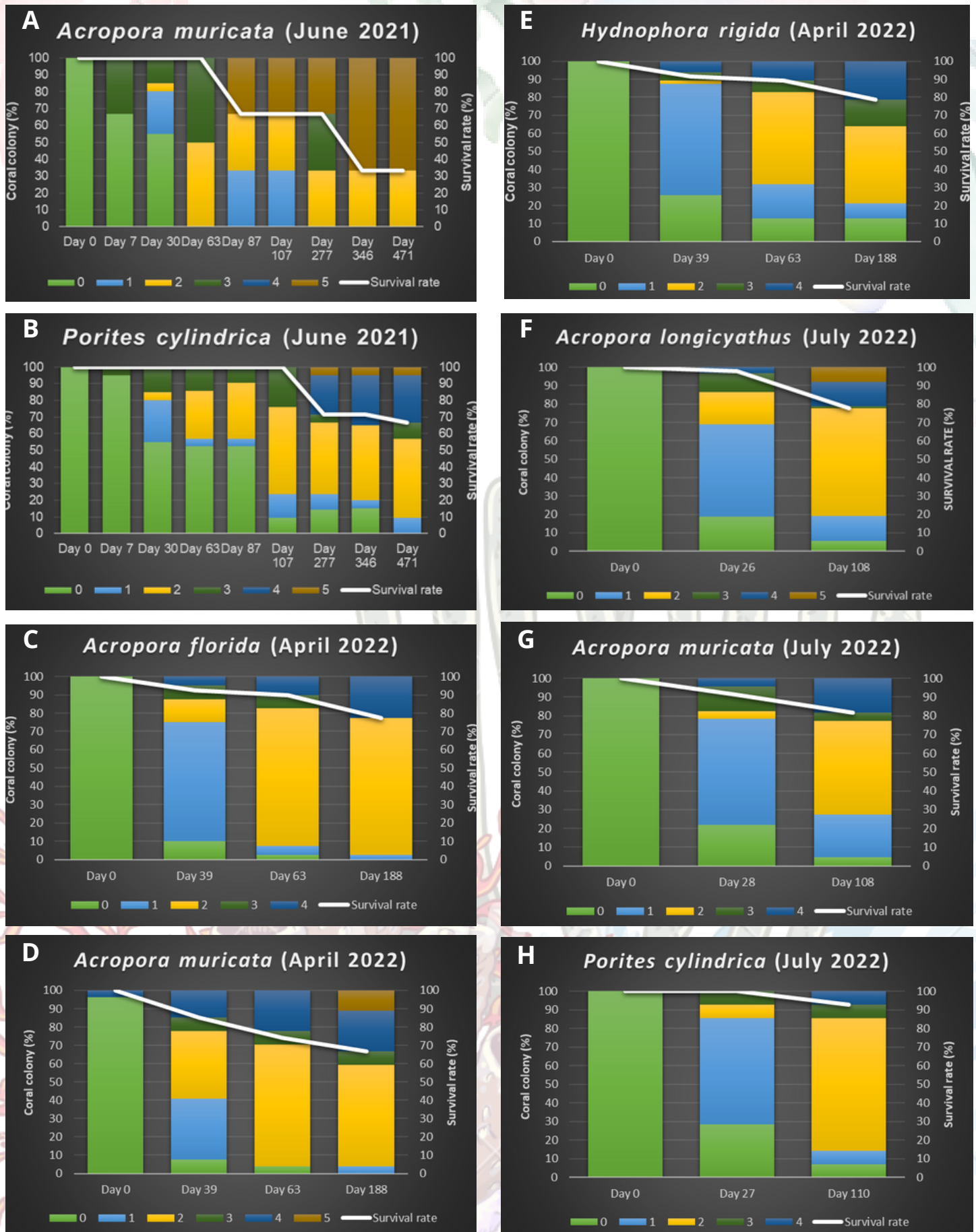
Figure 22. The attachment and survival rate of different coral species by batch in the natural reefs since June 2021 (A–B), April 2022 (C–E) and July 2022 (F–H). Note: 0=Non-attached; 1=Tissue sheeting; 2=Self-attached; 3=Attachment method failed; 4=Detached; and 5=Dead.
